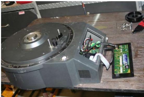
The front plate has 4 small Allen head screws holding it in place then the connector wires unplug from the main boards.
