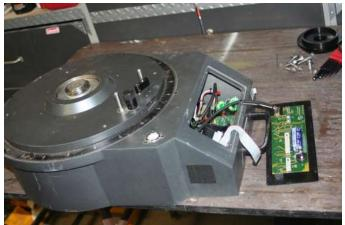
I started with the removal of the old components. First the Clutch and motor from the upper Fork (still attached to the OTA) The clutch simply unscrews and is removed
