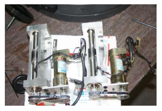
First remove the pulley and drive belt then remove the 3 screws holding the motor to the assembly.
